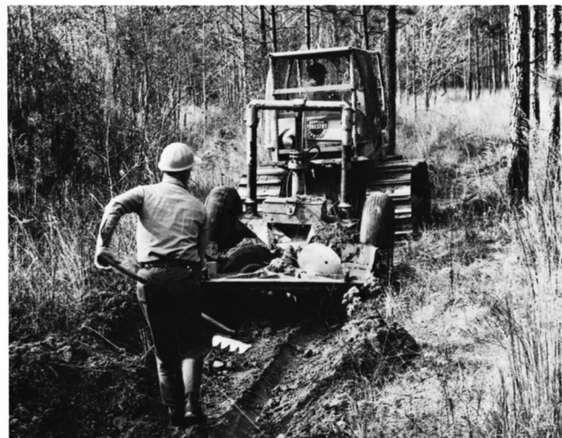
Figure A-5-2.2(b) Tractor plows are often used in suitable terrain to build firelines along the flank and rear of a wildfire.
